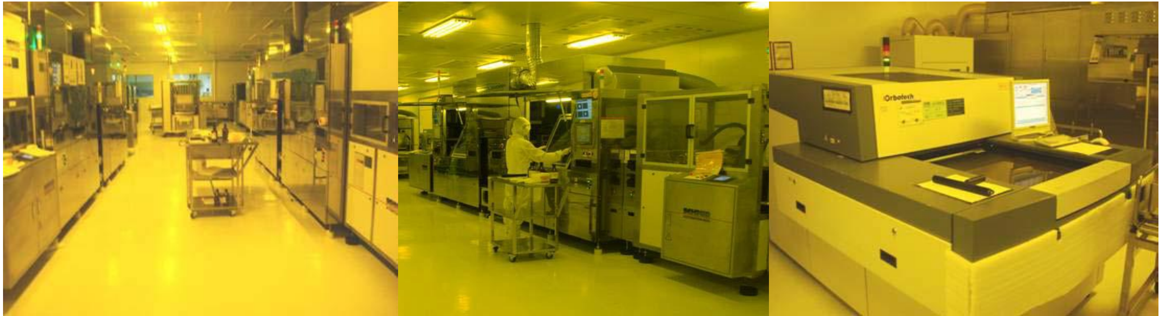
Class 1000 Clean Room with Auto Alignment Exposure Units and LDI
