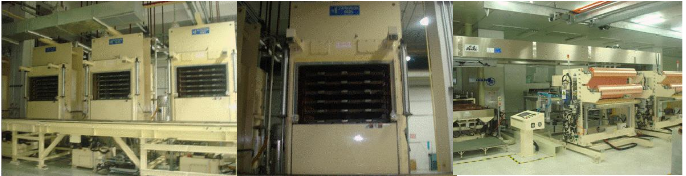
Automatic Lay Up and High Capacity Lamination Press with Auto-Loading
